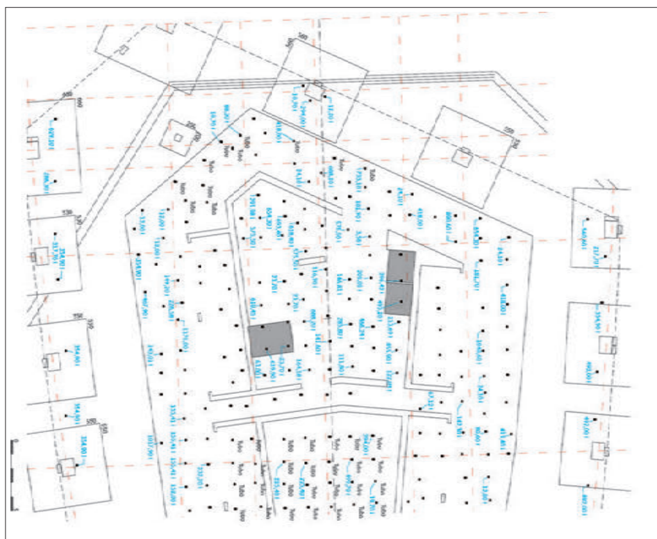
Figura 10 – As Built - Injeção - Ala B
